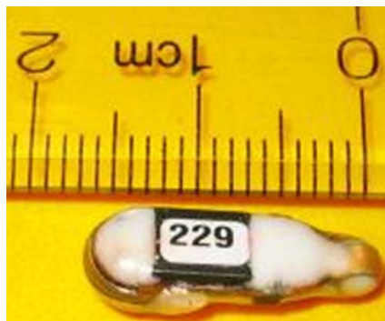
Figure 2.1. JSATS Acoustic Micro-Transmitter with Ruler for Scale
