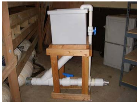
Figure 2.4. Release Apparatus for Turbine Intake 9C Releases at JDA in Spring
